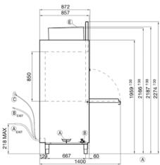
The IM1000 R commercial Utensil/potwasher with heat recovery is perfect for taking on even the biggest items in the kitchen, with its massive  $1320 \times 700$  baskets and 850mm high door opening it is guaranteed to take on the biggest jobs with ease.
